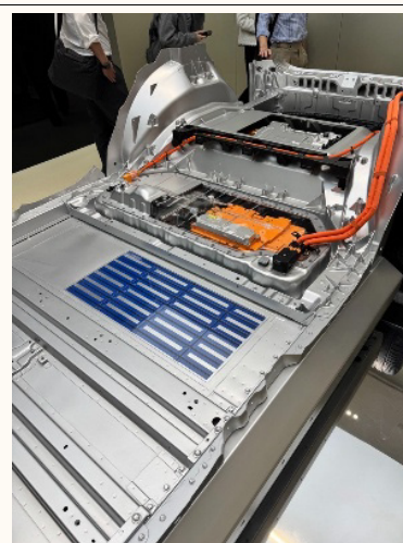
Figure 2: CATL EV battery system in a Xiaomi platform
